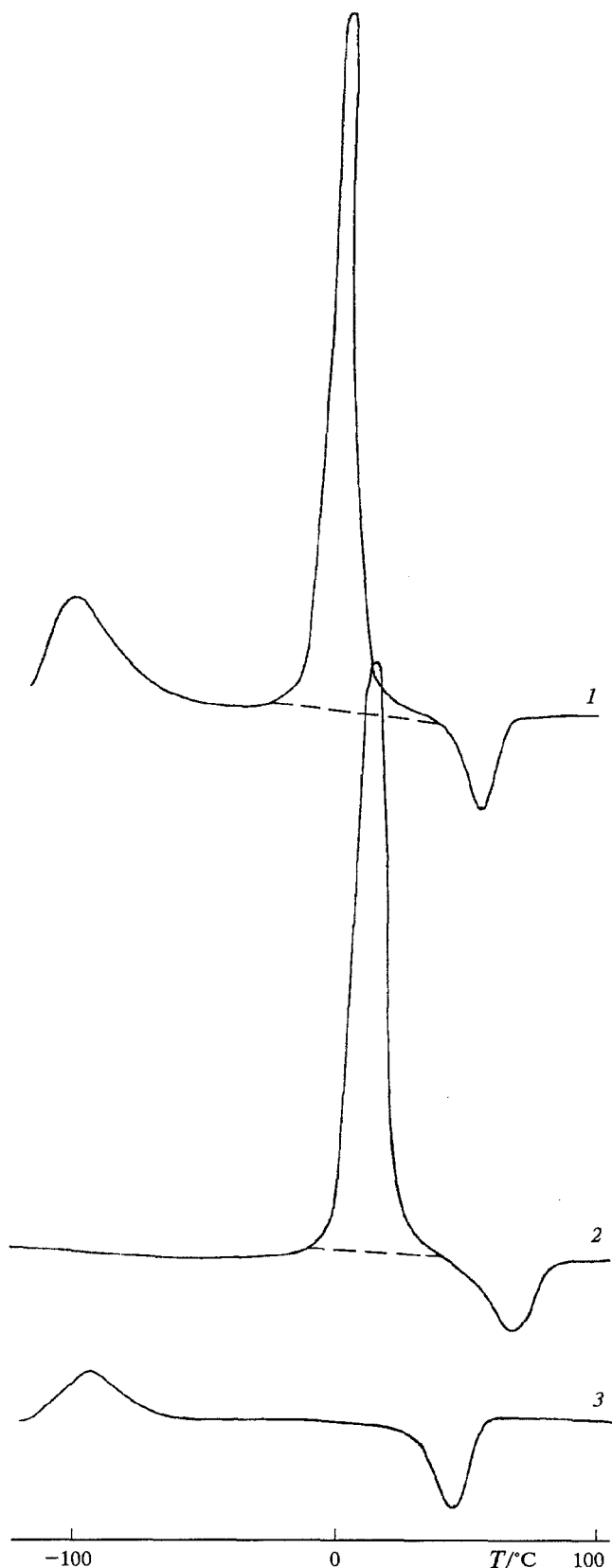
Fig. 4. TPR spectra of 5 % Pd/NaY catalyst: initial, pre-oxidized at 500 °C (1); oxidized with adsorbed H 2 O (2); after desorption of H 2 O (3).
